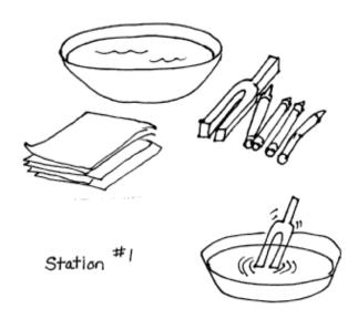
**Caution**: the resonating (fork) end of the tuning fork should *only* be placed in the water. Do not put the resonating end of the fork against the windows, eye glasses, or teeth. The tuning fork can shatter glass.
